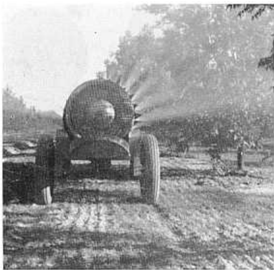
An air blast sprayer in operation to control Black Pecan Aphid in the Stahmann orchards of Santa Tomas, New Mexico.
