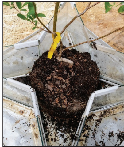
Figure 1. Horhizotron™ has four wedge-shaped quadrants that extend out from the root ball. Quadrants are constructed of glass panes connected by vinyl j-channels. The aluminum base onto which the glass panes are attached is fastened to a treated wood frame.
